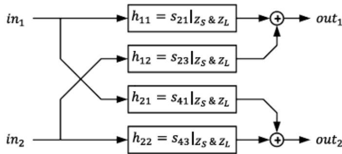
Figure (3) Thru and cross-coupled transfer functions of the MIMO channel
