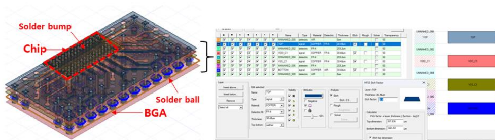
Figure 23. PCB/PKG CAD file Import, Structure and Stack-up parameters assign
